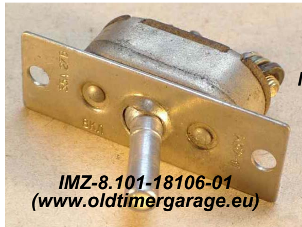
Masseschalter (Ground Switch)
