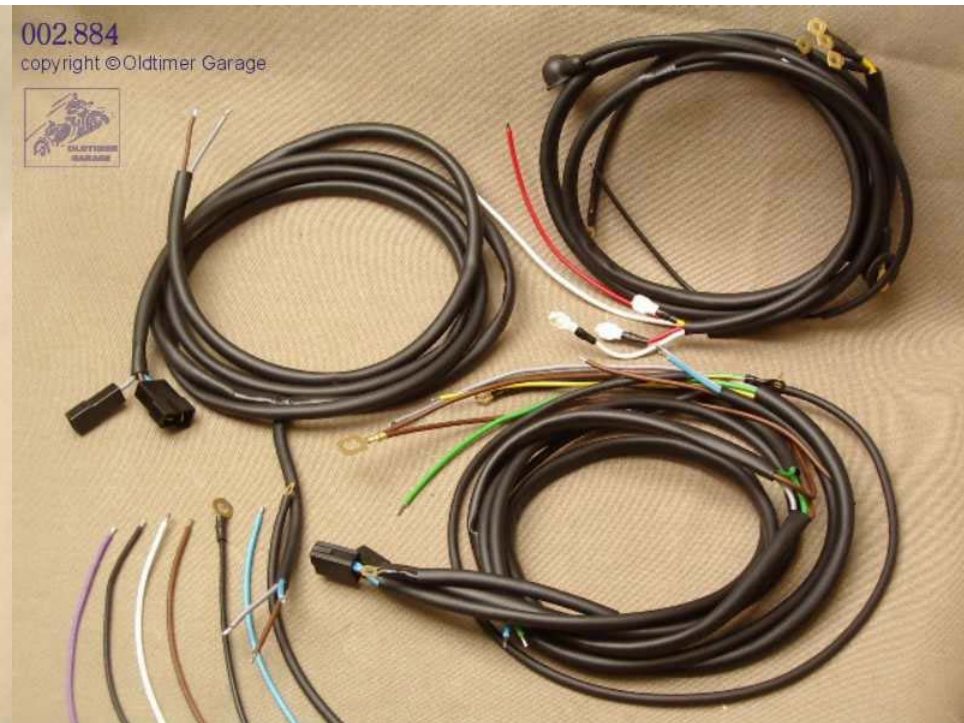
Wiring for K-750, MB-750, MT-12 with optional neutral switch and electronic regulator
