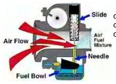
Fuel and air flow into and mix together in the carburetor, a process critically dependent upon the dimensions of all the ports, channels, jets, passages, chambers, etc., therein. Any contamination, any foreign
