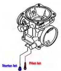
provides an opportunity for removing anything on the interior float bowl surface, a source of potential future problems. When finished, button 'er up, righten up the carb and tighten the fore and aft hose clamps, close the dump screw, and turn on the fuel petcock. Any luck? If not, we've gone just about as far in the cleaning department as possible without carb removal and disassembly. Advance (or retreat?) to the next section!
