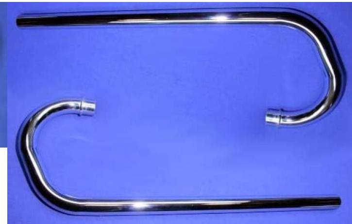
Downpipes, SS, Extra Long (approx. 130cm) (Side Valve: M-72, K-750, BMW R71) Often used without mufflers, ending at the rear of the rear wheel. Result: deep and full sound! Because of the length the riding is relative quiet, but at standstill indescribably nice. Vendor ID: S4680 List Price: €175.00 pair (www.ural-zentrale.de)
