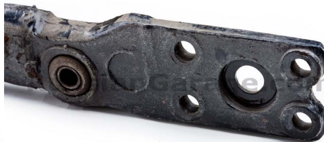
Silent-Block, 32mm OD, 13mm ID, height 29mm Vendor ID: 332 List Price: $3.00 ( www.russiagarage.com )
