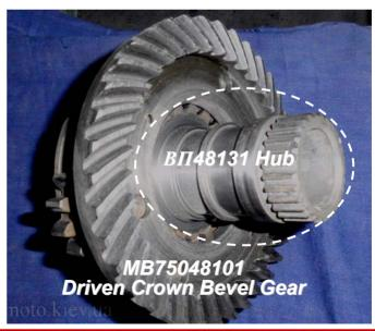
The inner workings of the MT-16 differential show the idle and satellite gears, the crown gear and the hub.
