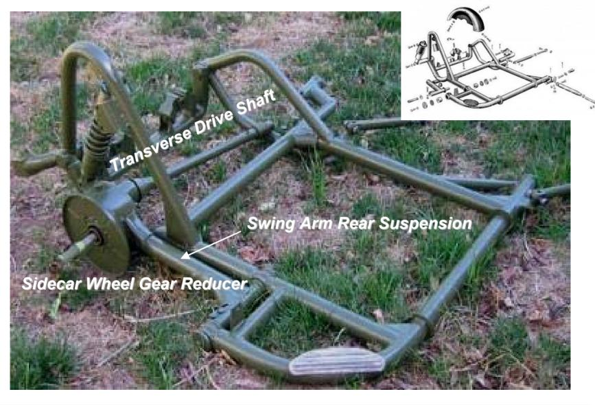
The bare sidecar frame shows the transverse drive shaft connected to the gear reducer, which drives the sidecar wheel.
