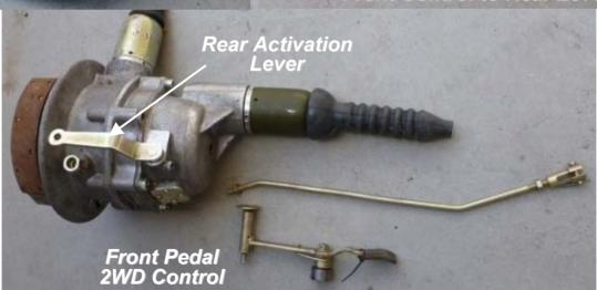
The locking mechanism from Oldtimer garage is a differential lock that is easy to install on the Dnepr MT-16 full-time 2WD (with differential), giving the possibility to lock the differential, just like an off-road motorcycle. The only work required is drilling/milling two holes in the right cover on the FD.
