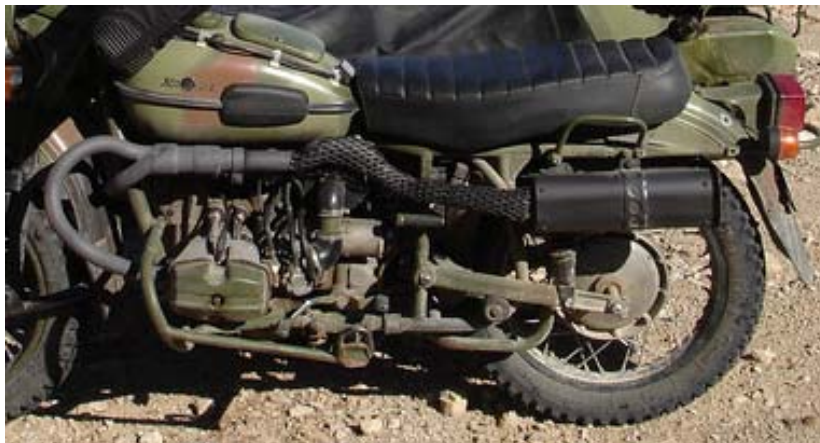
For V3.2, Headers Are Same Length and Uses FMF Muffler. Worked Very Well, but Wanted Something Simpler and Lighter.
