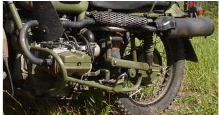
For Version 2.0 Headers, As Well As Muffler Elevated, Using the Same Kawasaki Muffler. Worked Well, So Decided To Make a Better and Lighter System.
