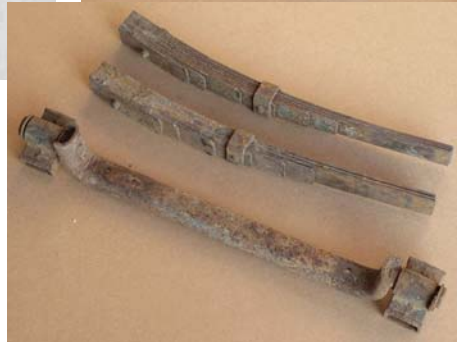
Leaf-Springs with Holder (M-72, Ural M-61, -62, -63) Vendor ID: 003.574 List Price: €75.00 Used ( www.oldtimergarage.eu )
