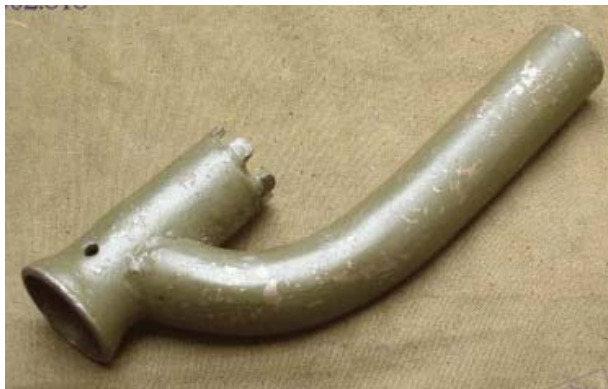
Sidecar Ball Joint (M-72) Part #: 7220075 Vendor ID: 002.818 List Price: €18.15 ( www.oldtimergarage.eu )
