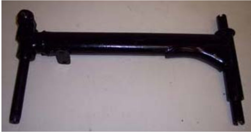
Sidecar Swing-Arm, For Models with Sidecar Brake, but Goes Well with Sidecar w/o Brake (K-750)
