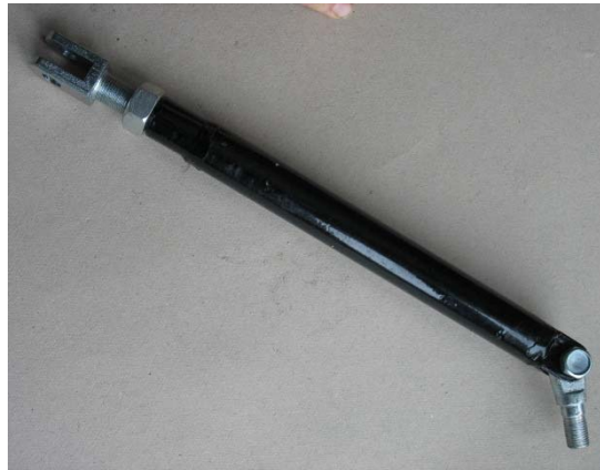
Sidecar Mount Set, Length: 300mm (MB-750) Vendor ID: 000.465 Part #: 650202 List Price: €32.26 (www.oldtimergarage.eu)
