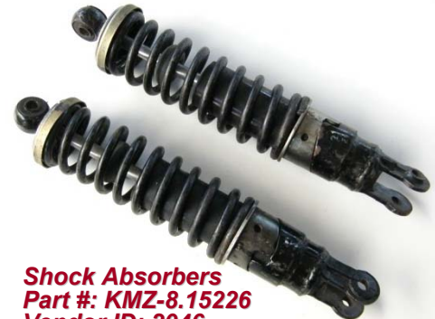
Shock absorber, Chromed (Cr) (K-650/MT-8, MT-9, MT-10, MT-11, MT-16, Ural 650) Part #: KMZ-8.152 26001-06 (black) Replace Part #: 5309300A Length: 355 mm between bolts List Price: €49 (www.henriksson.ee)
