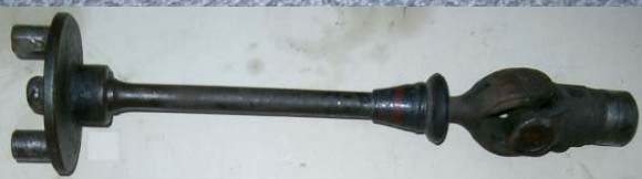
Final drive shaft (cardan shaft), Cr With joint for M-72 and some Dnepr and Ural models Overall length: 41cm Final drive shaft, chrome-plated Vendor ID: S872-KUE List Price: €59.89 ( www.ural-zentrale.de )
