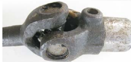
Coupling for Sidecar Drive (Thick Driveshaft) Vendor ID: 1212 List Price: €123.00 (moto-boxer.com)
