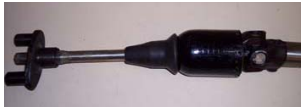
Propshaft with Universal Joint (K-750) Vendor ID: 176 List Price: €99.00 (www.ural-hamburg.de)
