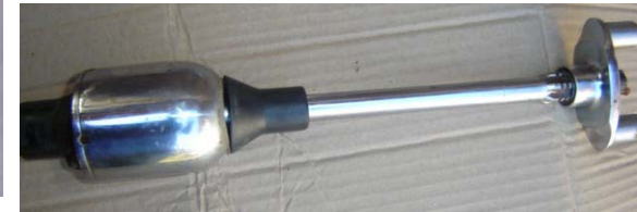
Propeller Shaft, Chrome (M-72, K-750, M-61) Vendor ID: 612 List Price: €69.99 ( russianspares.com )
