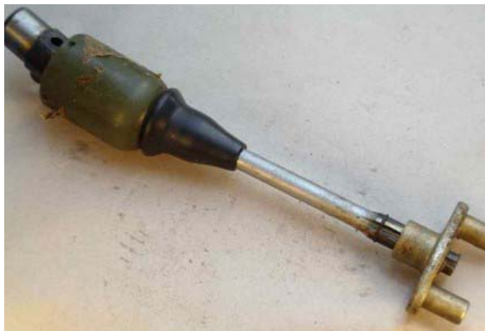
Cardan Shaft (MB-650, MB-750) Part #: MT905300 Vendor ID: 000.658 List Price: €126.02 (www.oldtimergarage.eu)
