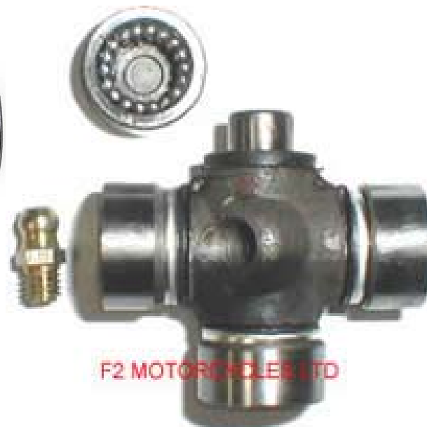
Universal Joint. This fits Ural M-72, M-63, M-66, M-67, 8.123, 8.128, Dnepr, K-650, K-750, MT-9, MT-10/6, MT-11, and probably all other Ural and Dnepr models. If you have play in the shaft drive universal joint this will fix it as long as the two outside forks are not worn. Comes complete with center cross, all needle bearings, seals and caps. You need to retain your original circlips. This is not exactly a joy to fit. Part - F21413 List Price: £26.00 ( www.f2motorcycles.ltd.uk )
