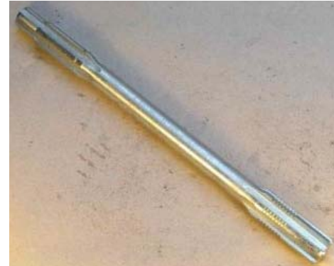
Cardan Shaft, Short (265 mm), Allows mounting Dnepr MT804 Reverse Gearbox in Short Frames Part #: 75005301-A Vendor ID: 000.654 List Price: €42.34 (www.oldtimergarage.eu)
