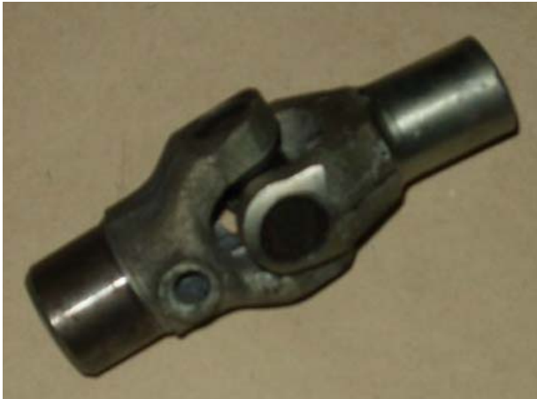
Cardan Shaft Hinge (MT-11, MT-16) Part #: 75005310 List Price: $58.00 ( www.dnepr-kiev.com )
