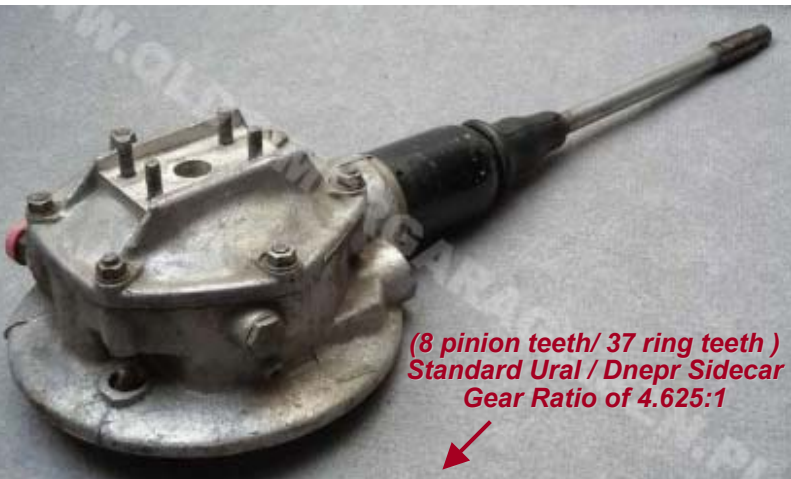
Rear Drive with Cardan Shaft, 8 X 37 Gear Ratio (K-750) Vendor #: 002.706 List Price: €327.66 ( www.oldtimergarage.eu )
