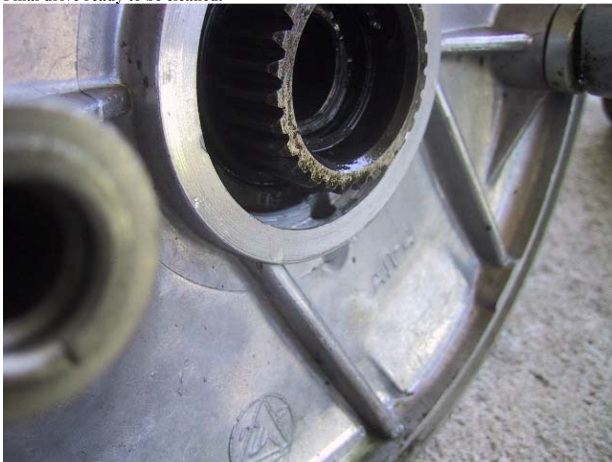
The little hole just below the wheel splines is the over-flow for the gear oil. If any oil should get past the seal it will trickle down this hole and coat your rear rim. Make sure it is not clogged with any crap.
