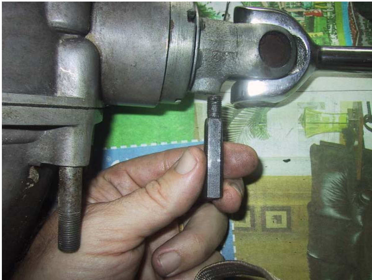
The wedge pin has two flat sides...
