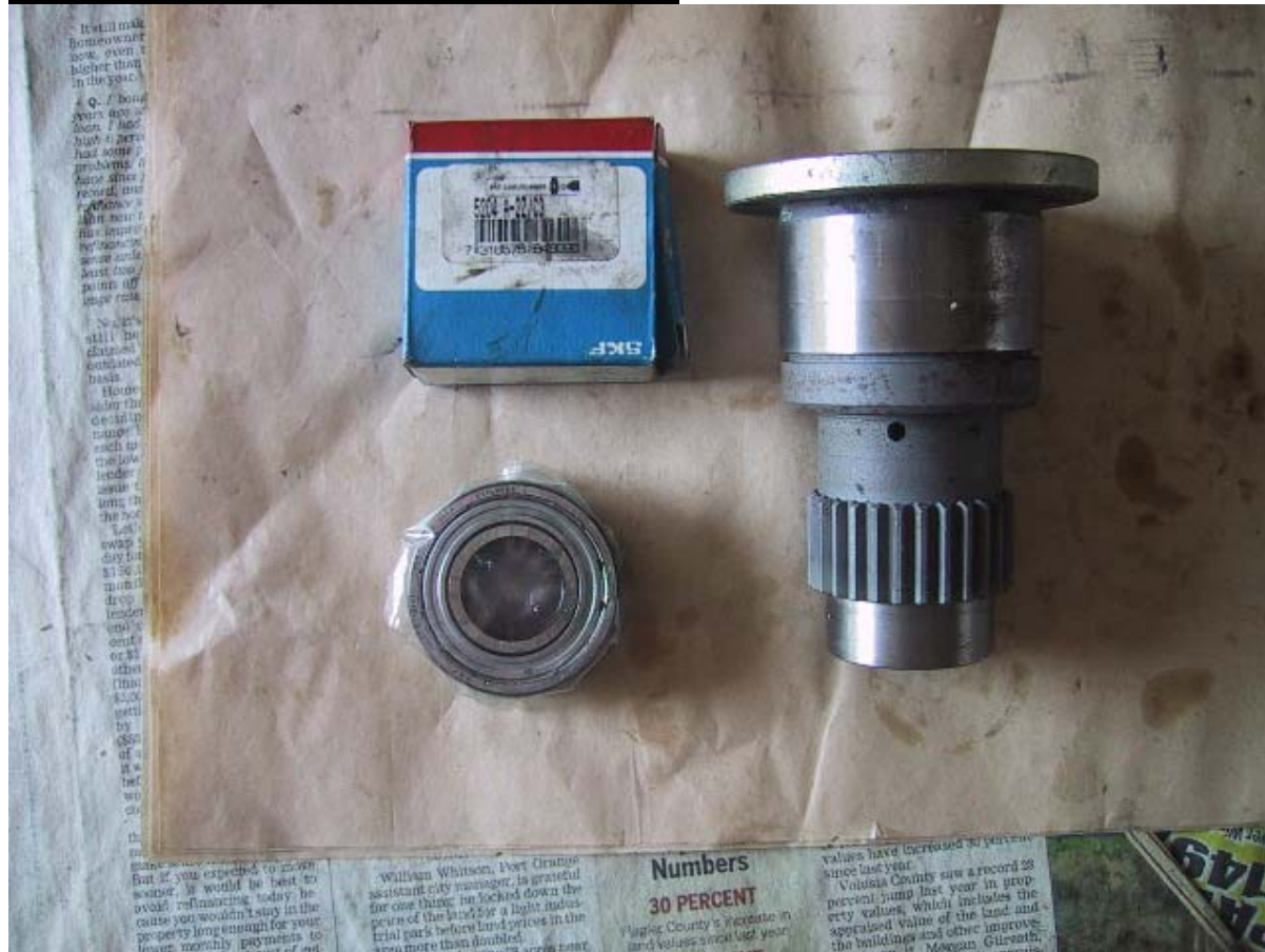
Splined hub and #204 bearing awaiting installation.
