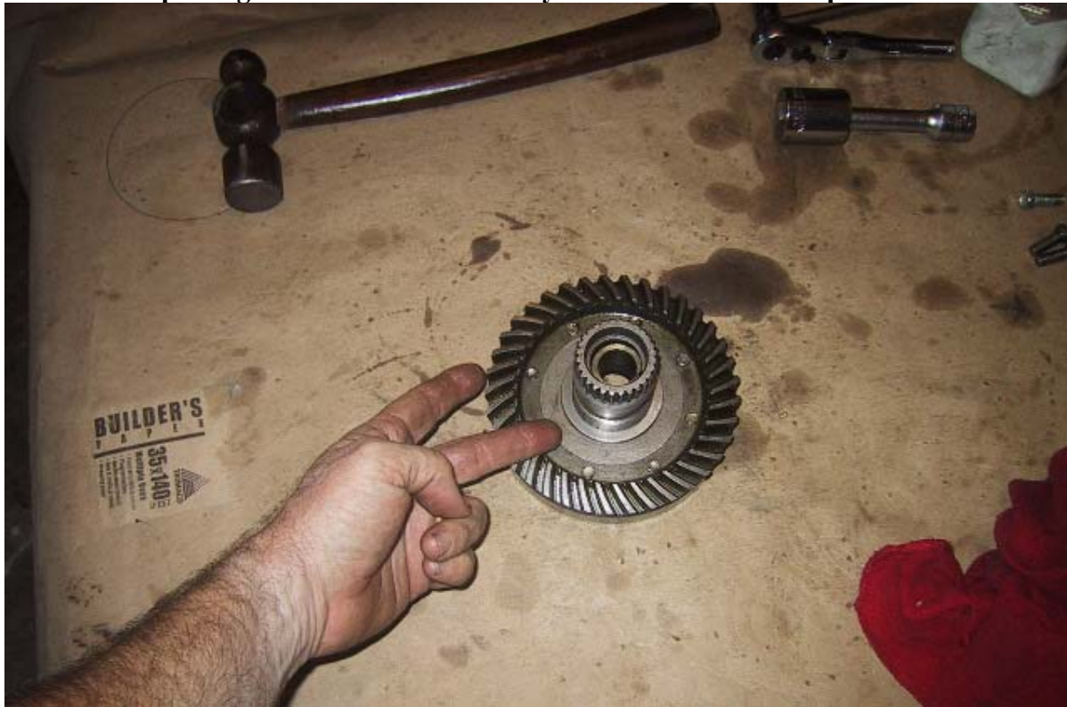
The steel spacer goes on second (hence the two fingers). There are 4 thicknesses of this spacer; 1.1mm, 0.95mm, 0.8mm and 0.65mm. These in conjunction with the final case gaskets are used to set the gear lash between the ring and pinion gears. This will be discussed further in 7.9(i) below.
