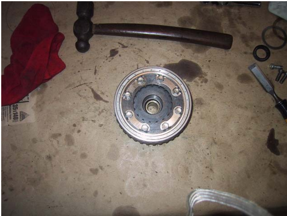
Spacer is in and the 22X40X10 seal is ready to install.
