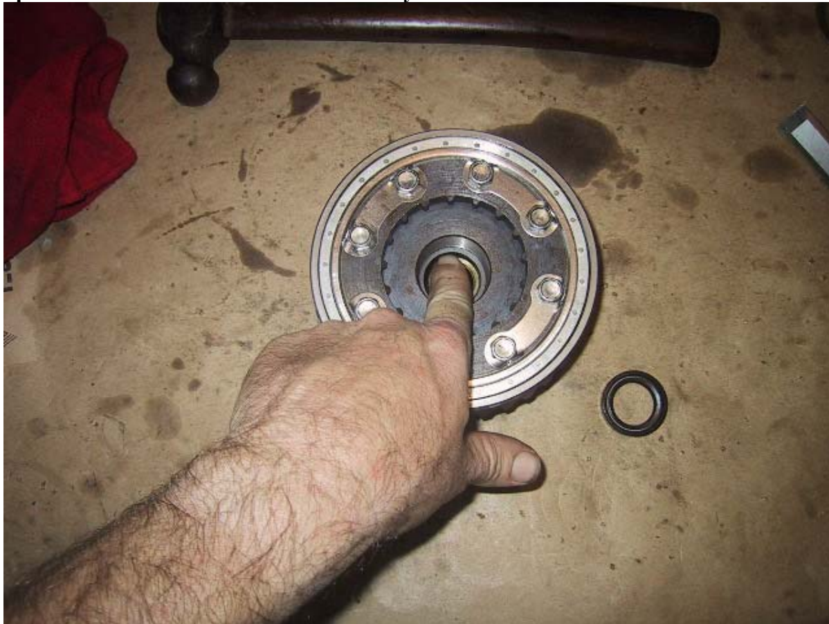
The seal needs to press down to this lip inside the channel.
