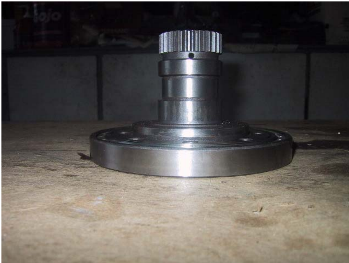
Side view of driven gear hub seated in bearing.
