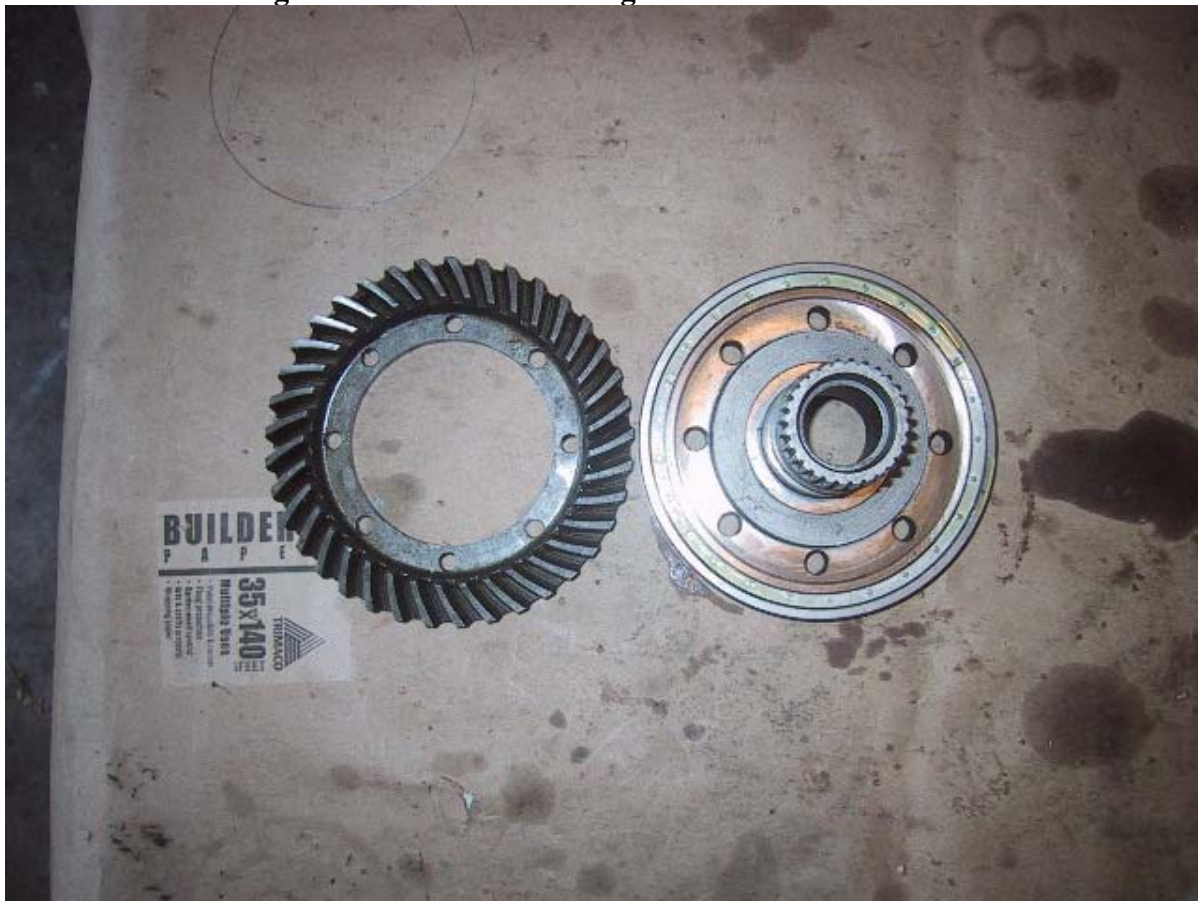
Take the ring gear and place it on top of the hub assembly. Take care in aligning the bolt holes. A couple of light raps on the floor should be enough to seat it.
