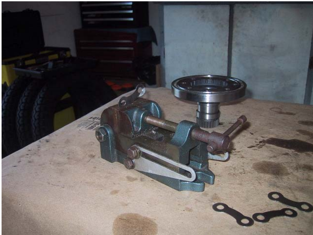
It is easier to pre bend the ends of the washers in a vise. Bend them up approximately 45 degrees.
