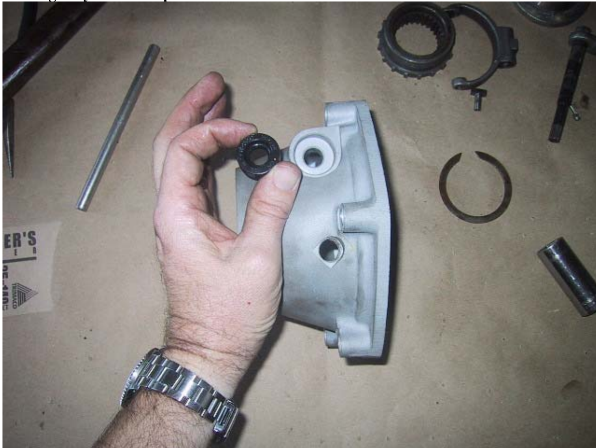
Now the 25.1 X 12.3 X 7 seal can be installed.
