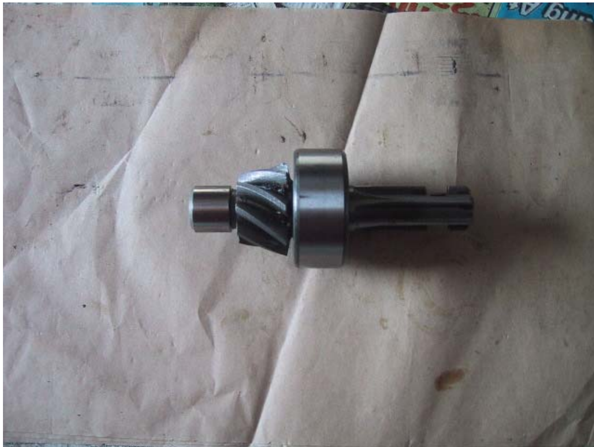
Three views of the assembled pinion gear, side...
