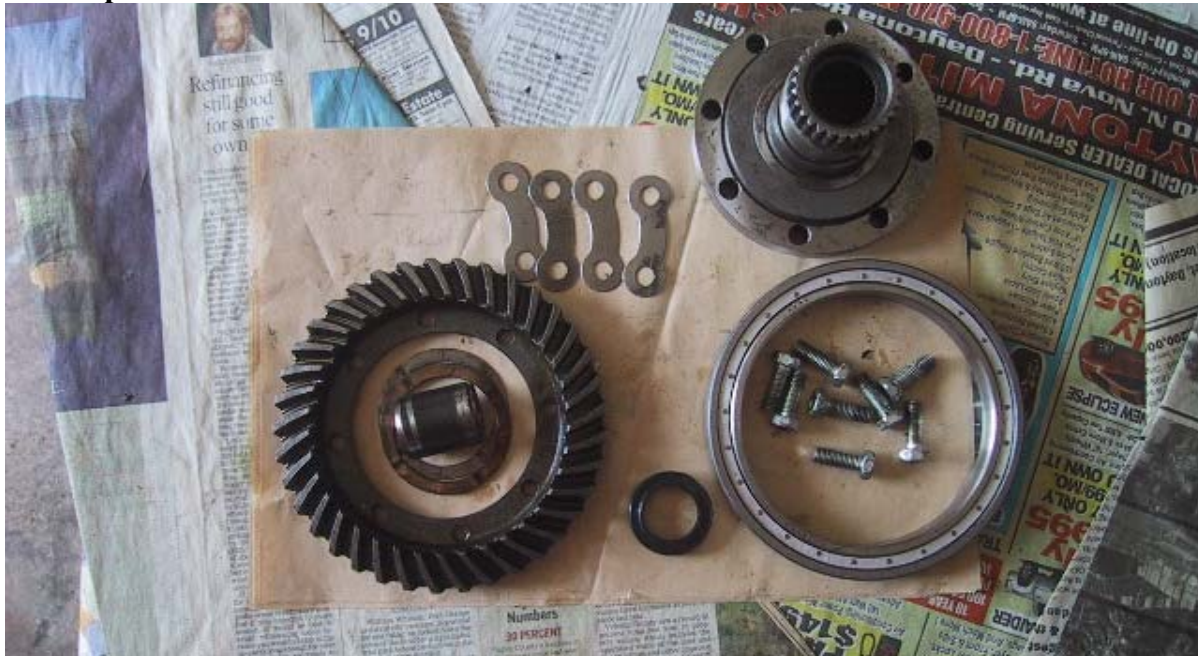
All the new parts needed for assembly. Driven gear hub, half moon lock washers, ring gear, shims, spacer, 22X40X10 seal, #1000822 (110X140X16) bearing and 8 M12 X 1.25 bolts.
