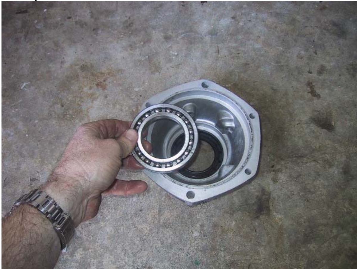
Next, place the #7000111 bearing in the outer housing...
