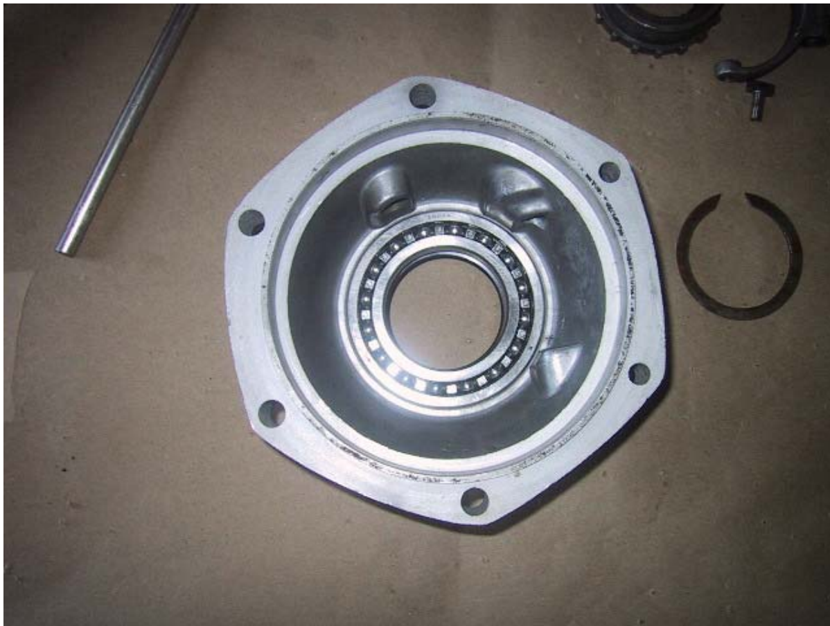
Bearing fully seated atop seal.
