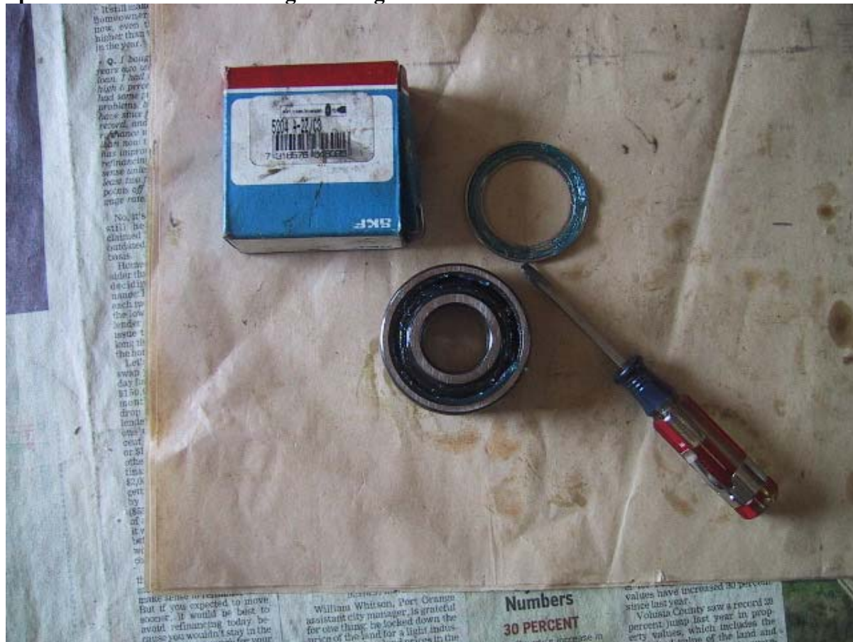
Once again, I remove only one seal from the bearing.
