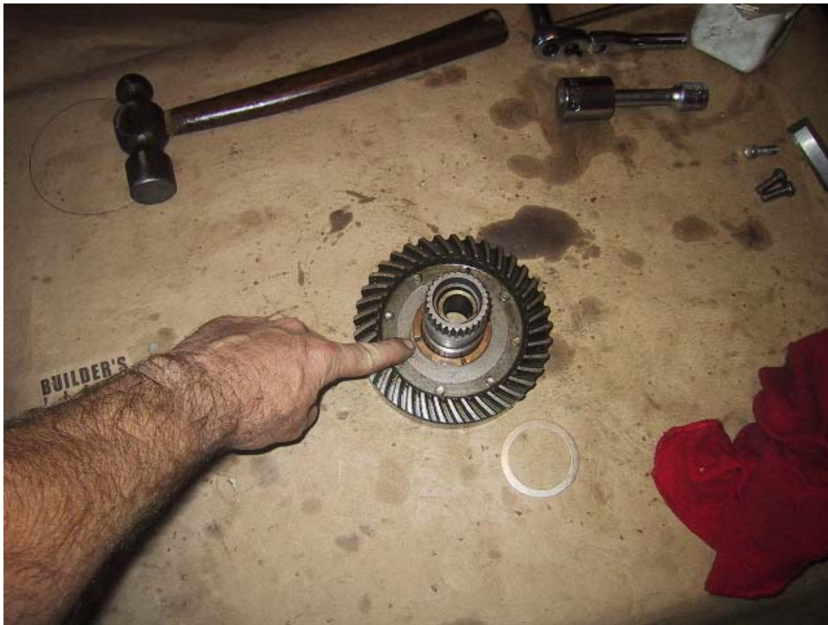
The bronze spacer goes on first. There is only one thickness of this spacer.
