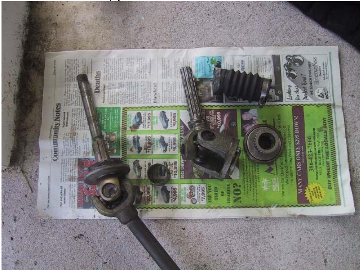
Clean the disassembled parts in your solvent of choice and inspect for wear. Replace bearings and worn parts as needed.
