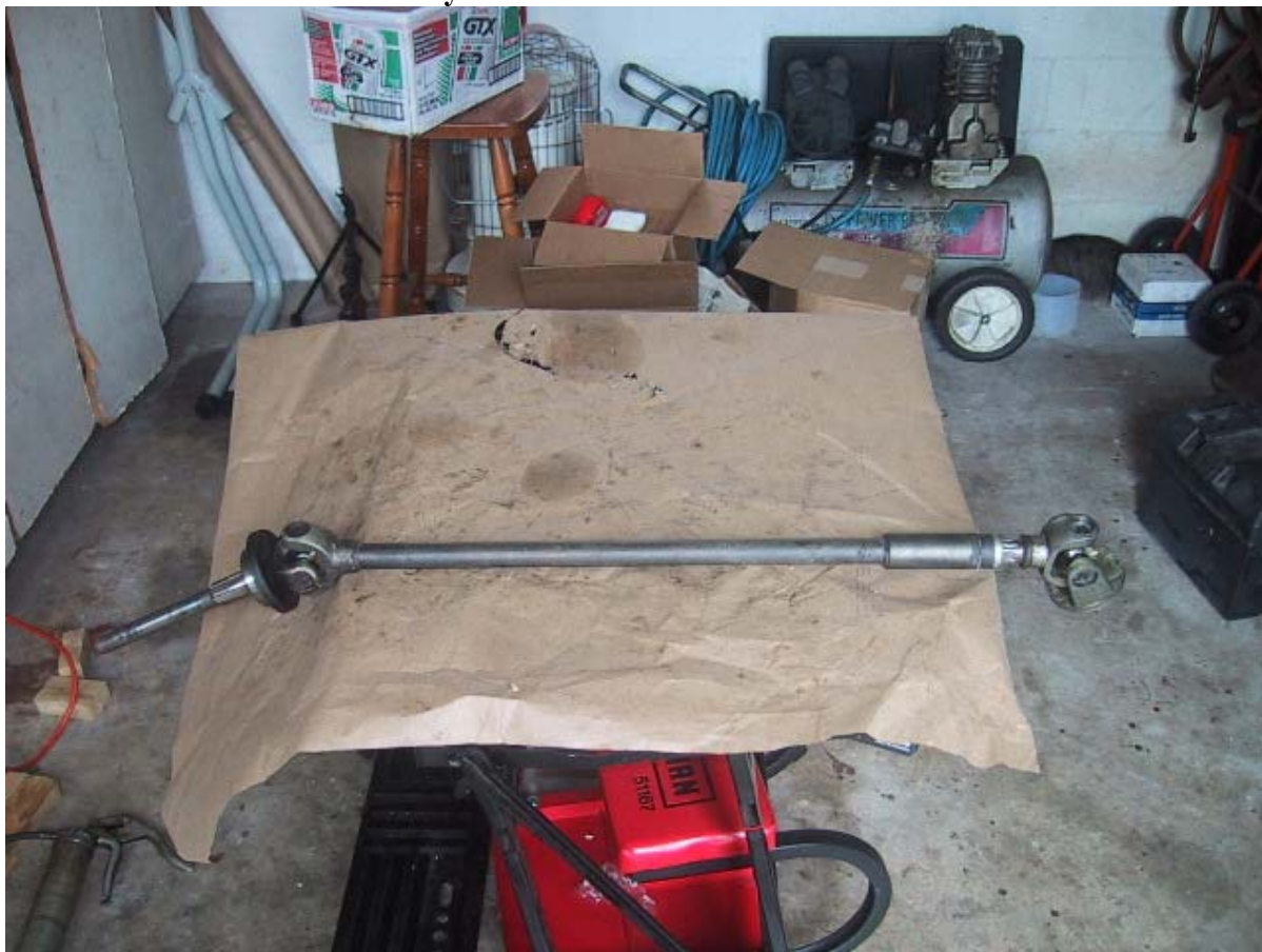
Here is the driveshaft laid out with the driveshaft fork assembly inserted into the driveshaft (right side). Make sure when you assemble the driveshaft on the motorcycle that the yokes are "in phase" or in alignment with each other. Note how the inside left yoke and the yoke of the fork assembly on the right are "mirror image" or matched to each other.
