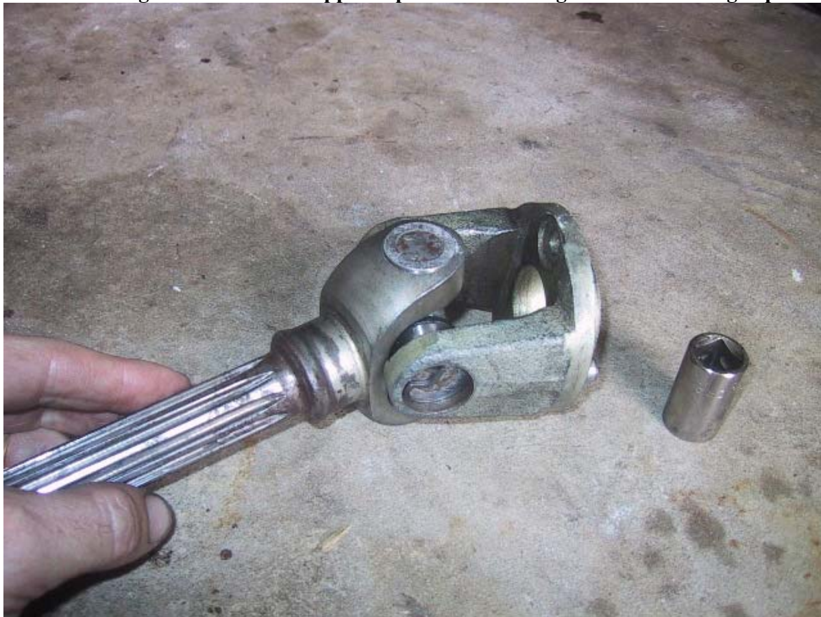
...flip the assembly over so you are looking at the flush cup....
