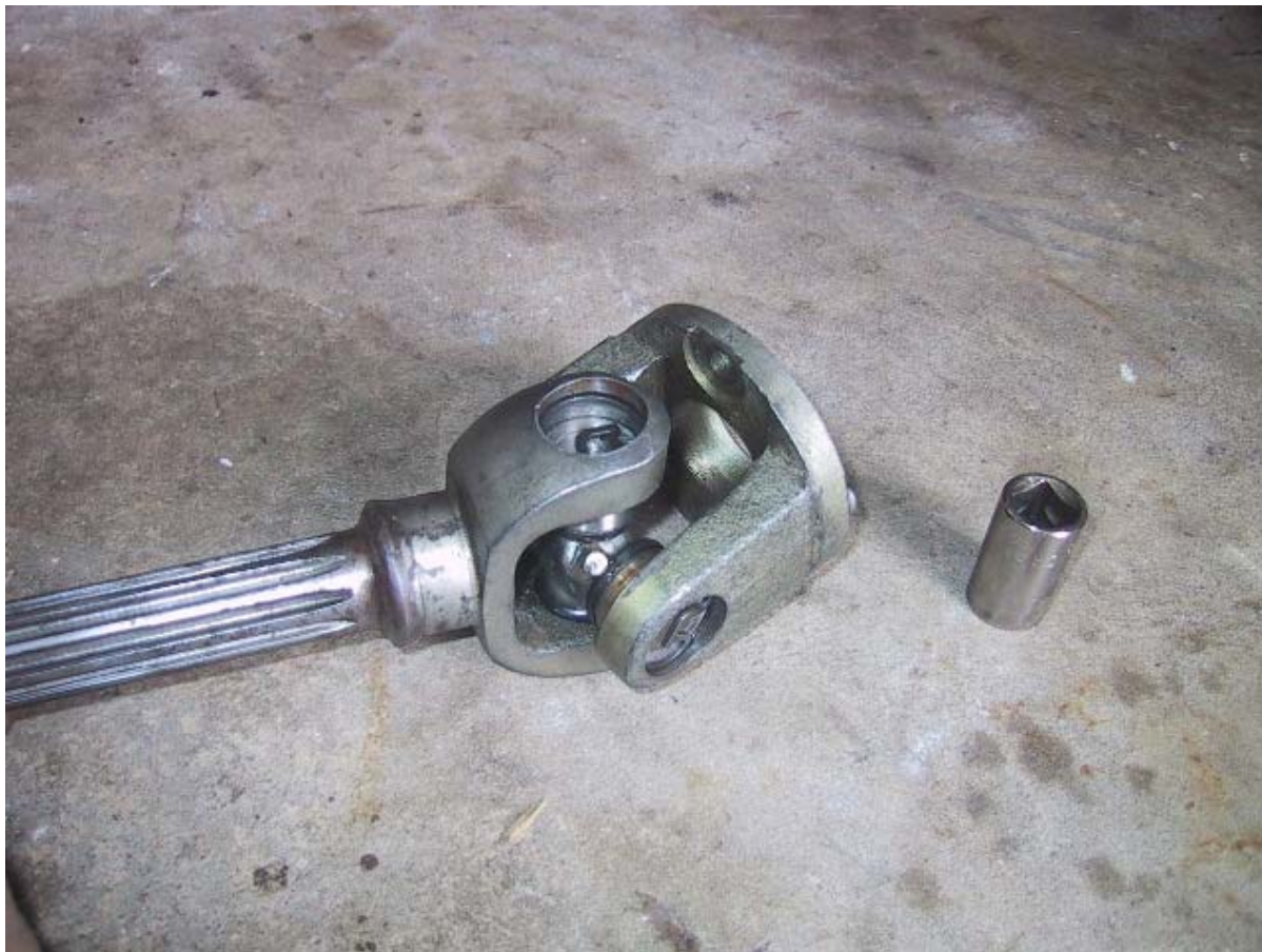
A view showing the zerk and the upper cup almost seated against the retaining clip...
