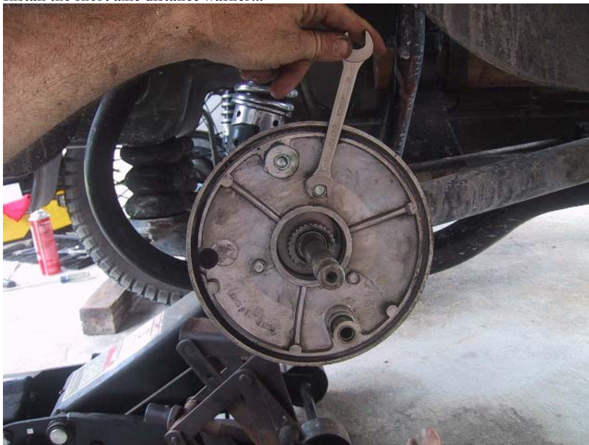
Use a 12mm wrench to install the 3 bolts holding the brake back plate to the wheel lever housing...
