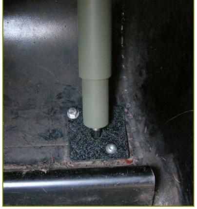
Moving to the inside of the tub, remove the right bumper bolt and set it aside, used later to anchor the foot plate. Just put it in to mark the second hole for now. Drill a 5/16" hole for the upper left anchoring point. Insert the bolt and tighten both hand-tight. Thread on the lower tube on foot plate.
