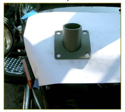
Next, install the upper tube so it fits up to the lower portion and square everything. Mark and drill the upper plate holes and remove the tube and paper. Clean up the holes and touch up with some paint to prevent rust. Some silicone sealant keeps out water on the top plate. Fit everything together and check that everything is square and snug. Re-tighten all bolts and you're done.
