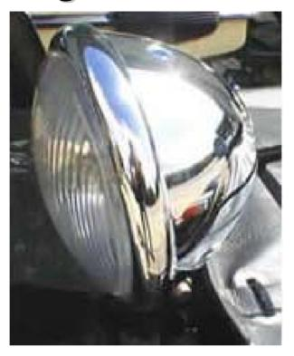
F2motorcycles offers an additional light on the nearside front of the sidecar. This is connected to the original Headlight and has both low and high beam and doesn't need to be operated separately using additional switches. Although the sidecar has a small white light on the mudguard, this additional hi/lo light makes it easier for on coming traffic to judge the width of the bike.
