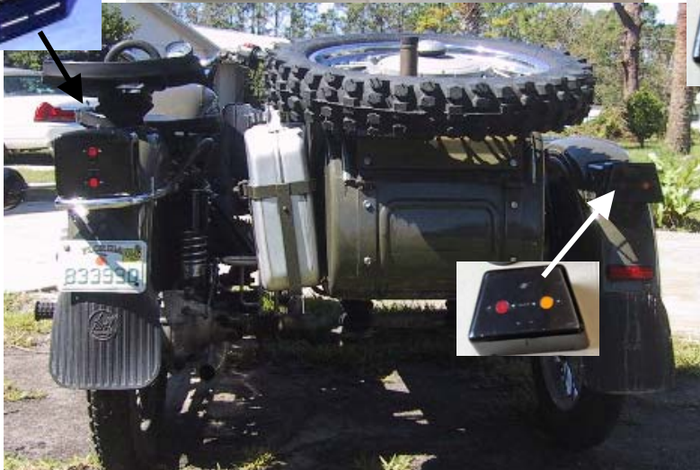
Tail light with license plate illumination and brake light (S1060)
