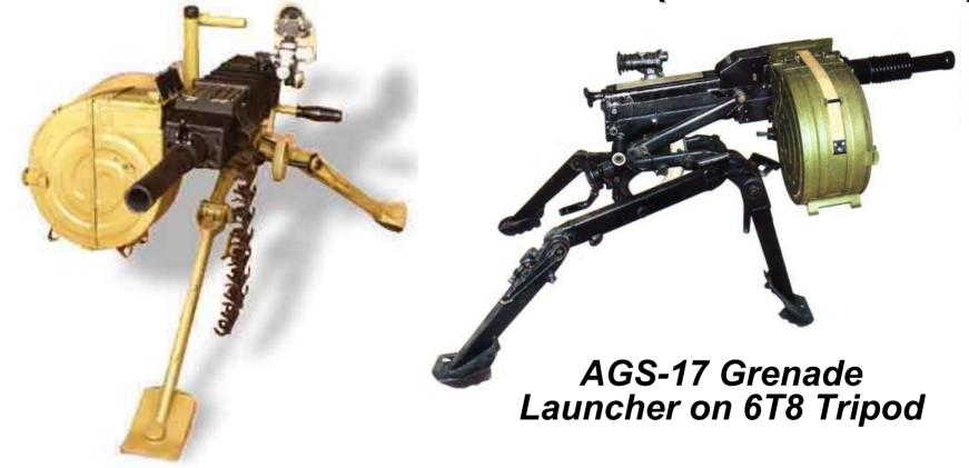
The automatic grenade launcher of the AGS-17 (40mm caliber) is one more arms type you can use with the Gear-Up. The AGS-17 (Avtomatischeskyi Granatmyot Stankovyi) Automatic Grenade Launcher is a heavy infantry support weapon designed to operate from a tripod or mounted on a vehicle. The AGS-17 fires a steady rate of 30mm grenades to provide suppressive and lethal fire.
