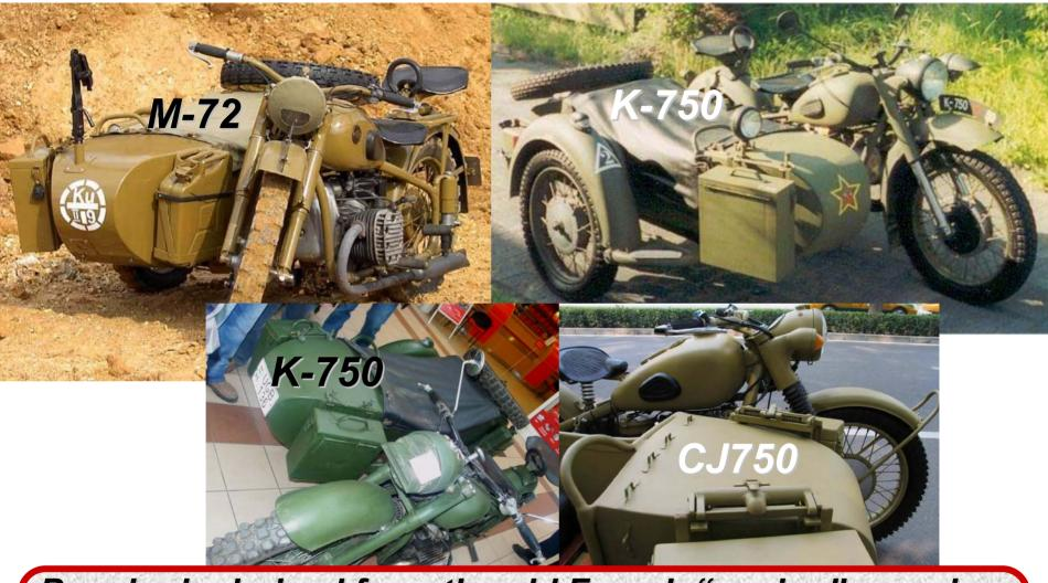
Pannier is derived from the old French "panier," meaning basket for bread. A Pannier is either of a pair of bags or boxes attached to the sides of the motorcycle or sidecar and is used to carry gear, clothes or tools.
