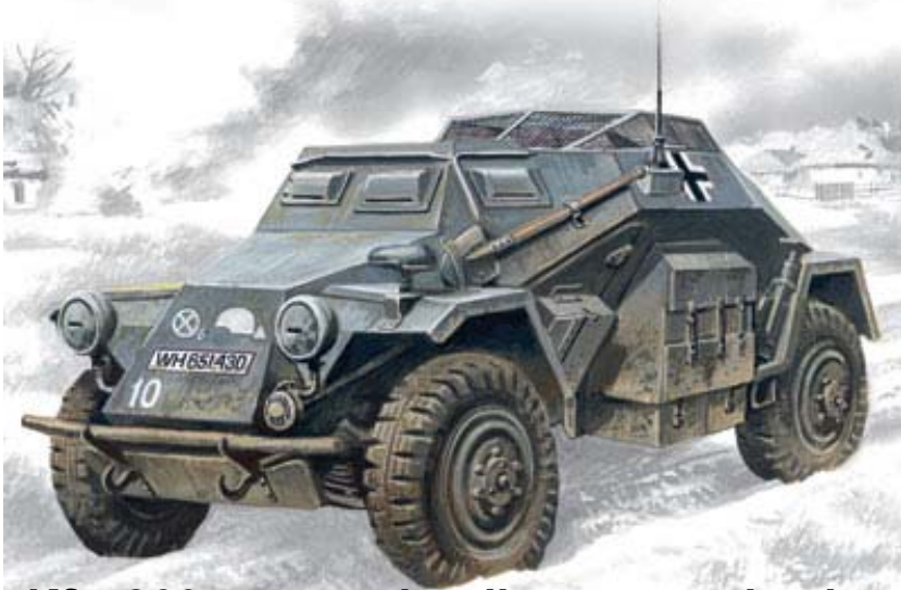
Sd. Kfz. 260 unarmed radio communication vehicle, used in tank and motorized units
