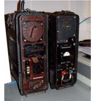
Feld.fu. b set (left), complete with flex antenna and battery charger (right)
