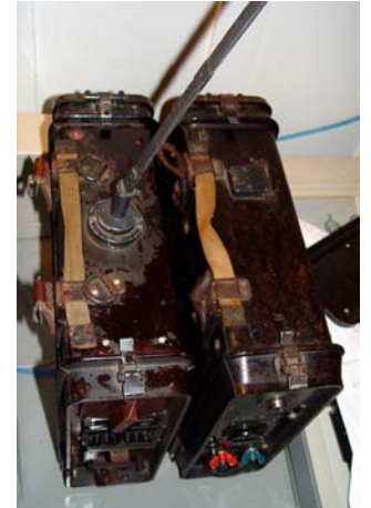
Feld.fu. b set (left), complete with flex antenna and battery charger (right)
