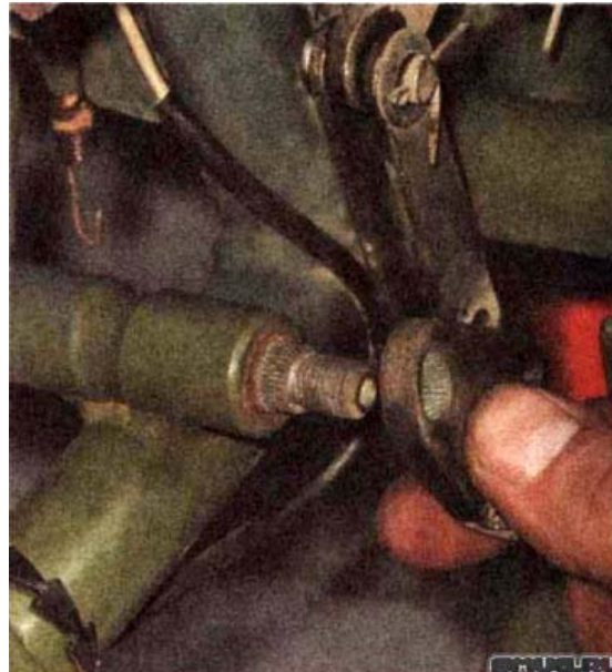
4. Use a wrench to remove the 17 mm axle pedal nut.
