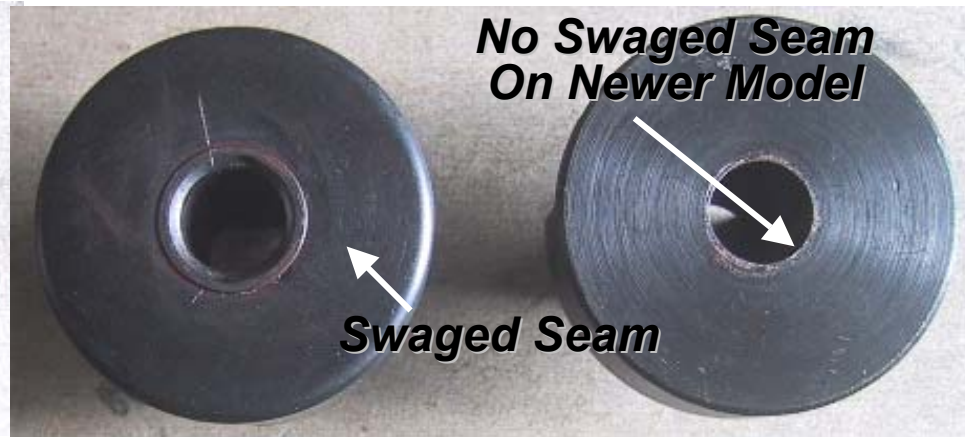
Left: Two-piece, with Swaged Seam on Back Right: One-piece; Devoid of Swaged Seam
