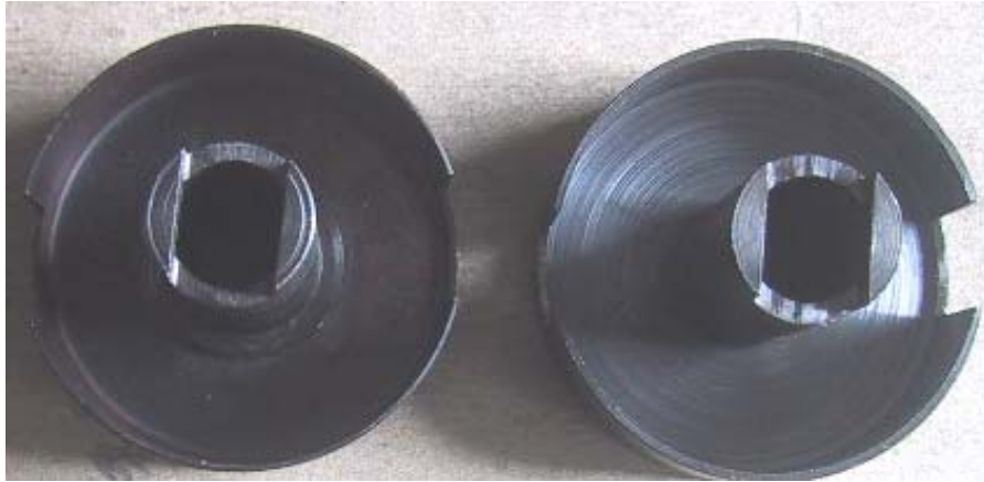
Left: Early-Manufactured, Two-Piece, Swaged-Joint Interrupter; Shoulder Meeting Round Skirt Right: Newer One-Piece, Machined Interrupter
