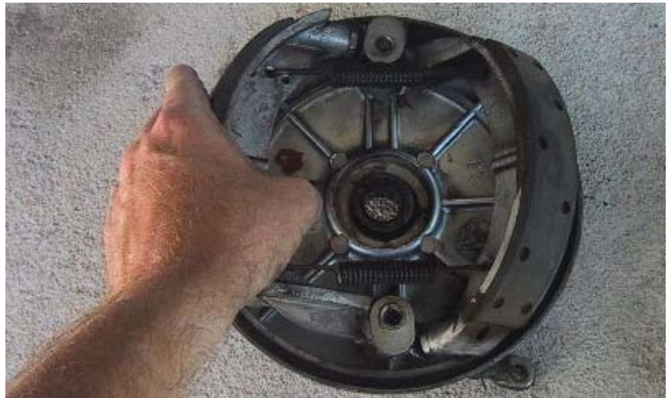
**To remove the brake shoes grasp each in the middle and pivot them up at the same time... *Note: Before removal, I use a scratch awl to mark the shoes "A" & "B" so they are put back in the original configuration.***
