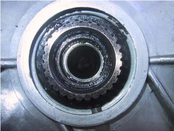
***Examine the final drive wheel hub splines for wear. If they are sharp and pointy it is time to rebuild/replace the splines. The splines above look brand new. Lightly grease the splines or the wheel hub splines before installing wheel.***
