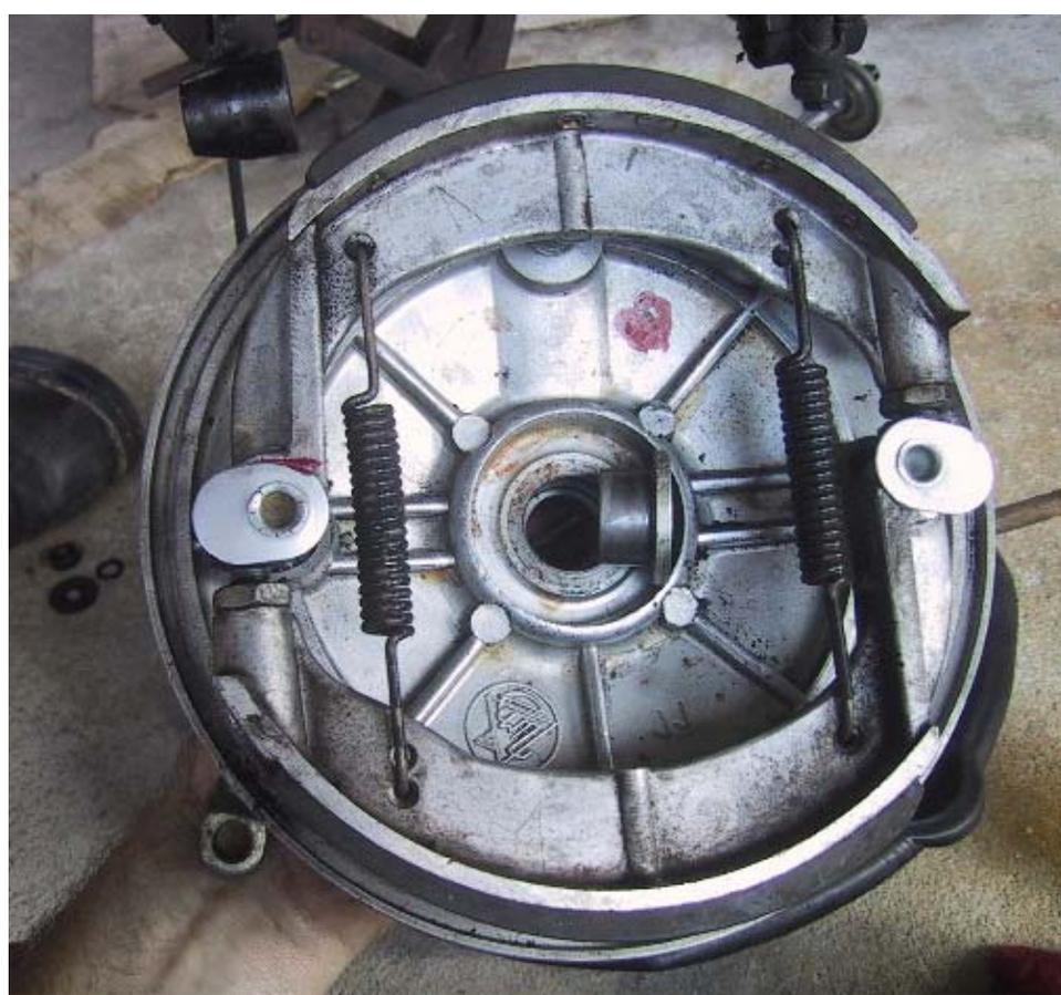
***Both are the same size and can go either position. A little grease keeps them from falling out. Put one on the inside...***
