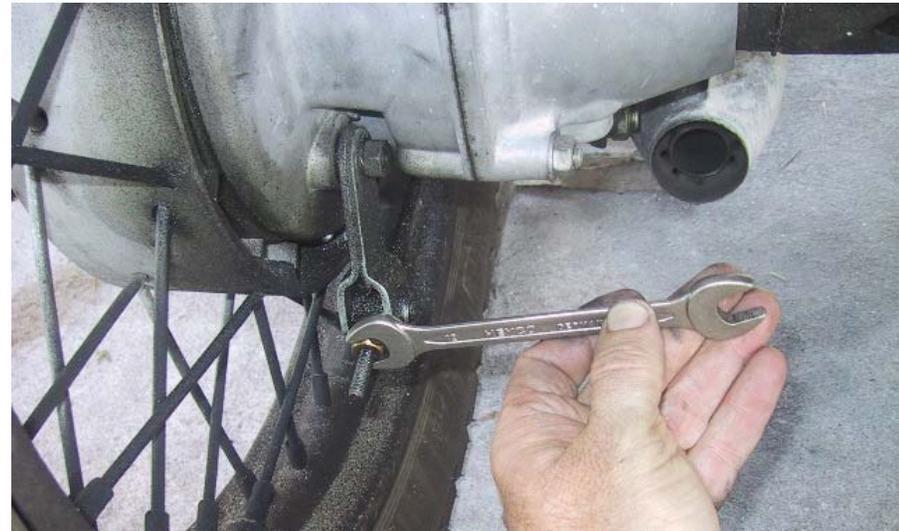
***Back off or remove the foot brake barrel-nut before remounting wheel.***
