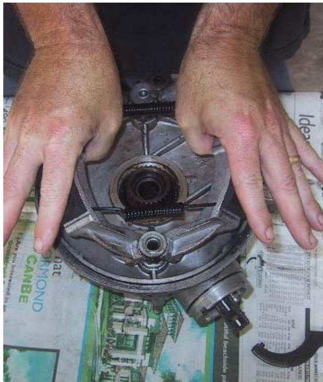
...and pivot the shoes upward against the cams.
