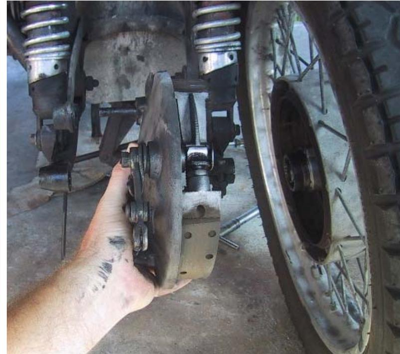
***...slip the brake plate off the torsion bar stud.***
