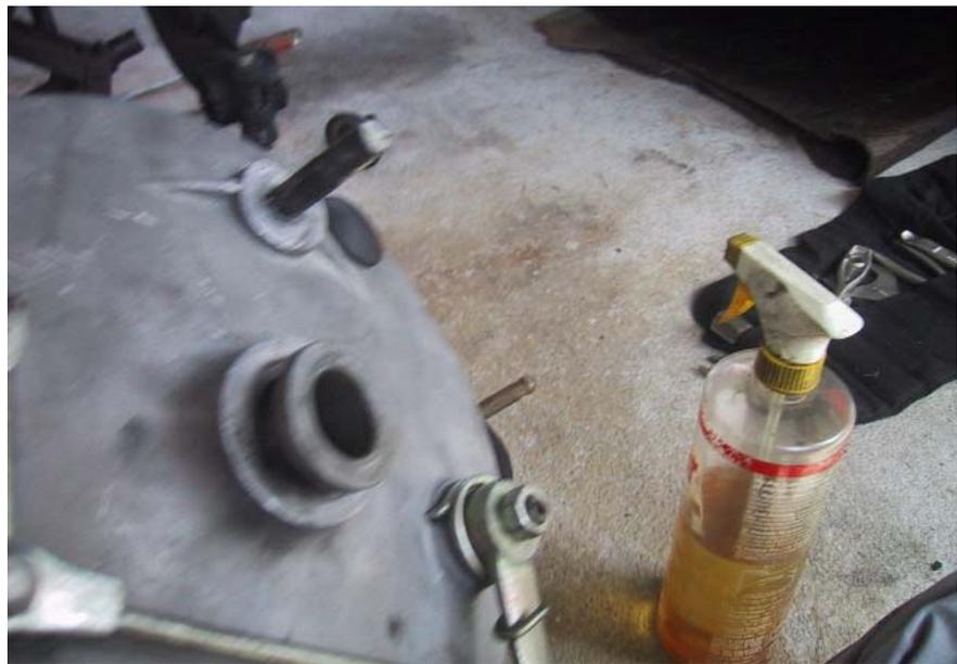
***...and one on the outside. You are now ready to slip the brake plate back on the torsion arm, mount the wheel, brake cable and adjust the brakes.***
