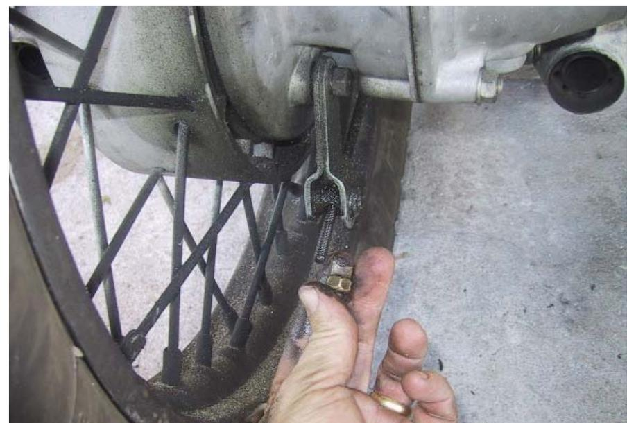
***If the nut is screwed in more than an inch or so; adjust the brake shoe adjustment bolt as shown in the "Front brake, Leading Link" section above to give yourself some more adjustment leeway.***
