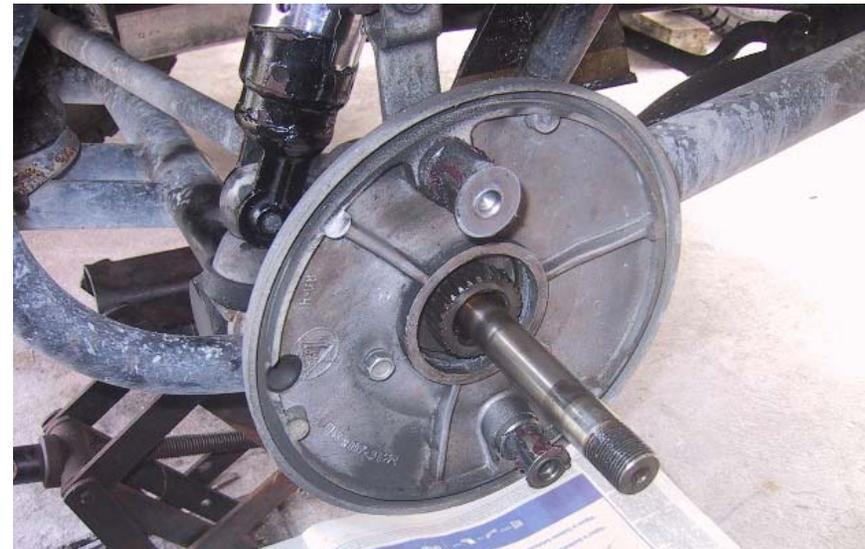
**...then grease the cams and axle before
