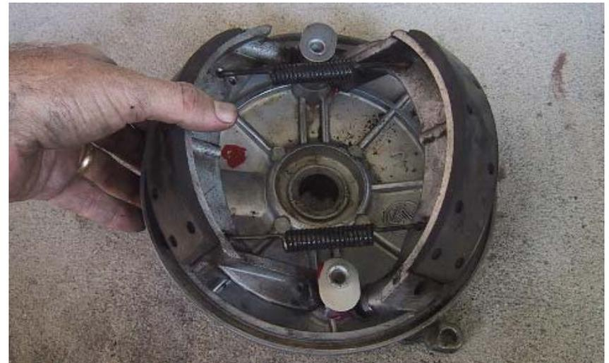
**Replace the shoes by folding them slightly in a "V", setting the contact surfaces of the shoes on the cams and pressing down at the middle of each shoe simultaneously. They will pop right on with maybe a minor adjustment to get them to click in.**
