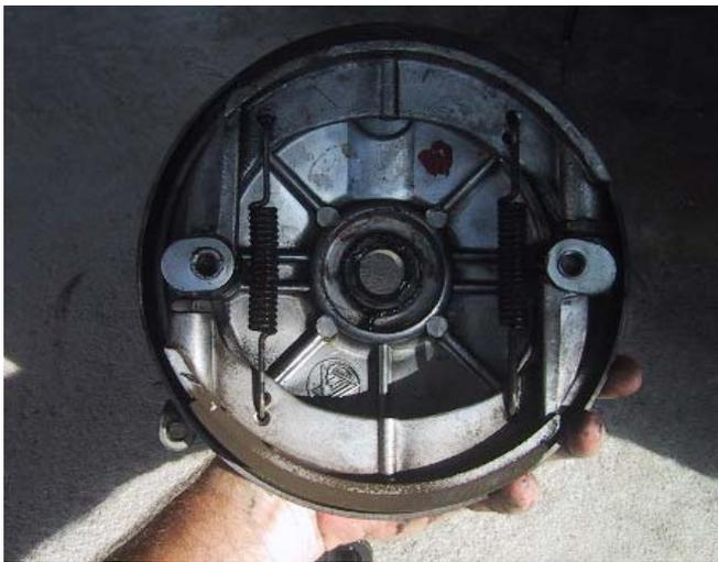
**The shoes are located top & bottom unlike the other drum shoes, which are fore & aft. It is a good idea to scribe a "top" and "bottom" or other mark on each shoe so they get put back in the same spot.**
