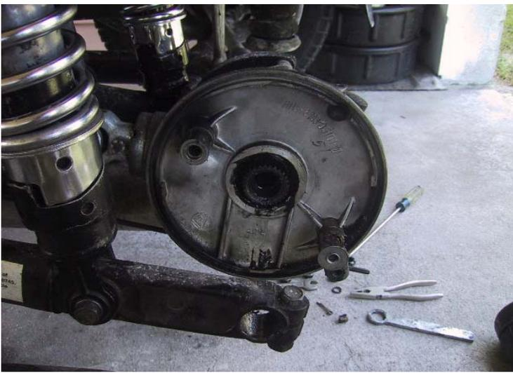
***Clean the brake plate and shoes with solvent of your choice. I use aerosol brake solvent or gasoline. Apply grease to the brake shoe cams and re-install the shoes.***
