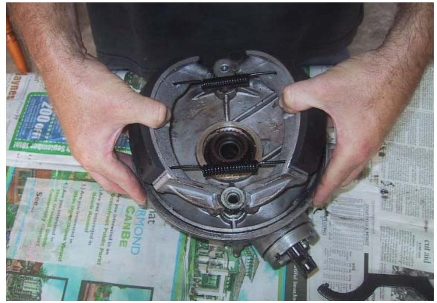
***When reinstalling the shoes; again grasp the middle of the shoe holding them in a loose "V", place the shoe-ends on their respective cams. Pull the shoes up against the top of the cams...***
