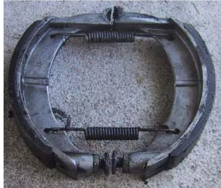
**Note:** Before removal, I use a scratch awl to mark the shoes "A" & "B" so they are put back in the original configuration. Remove the brake shoes by grasping each at the middle and pivoting the shoes up on the cams...
