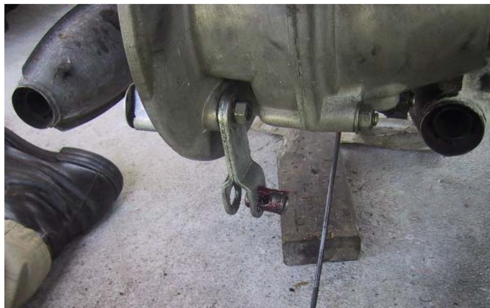
***Grease the barrel slide for the foot brake rod. Reassembly is the reverse order. Install the wheel and adjust the brake.***
