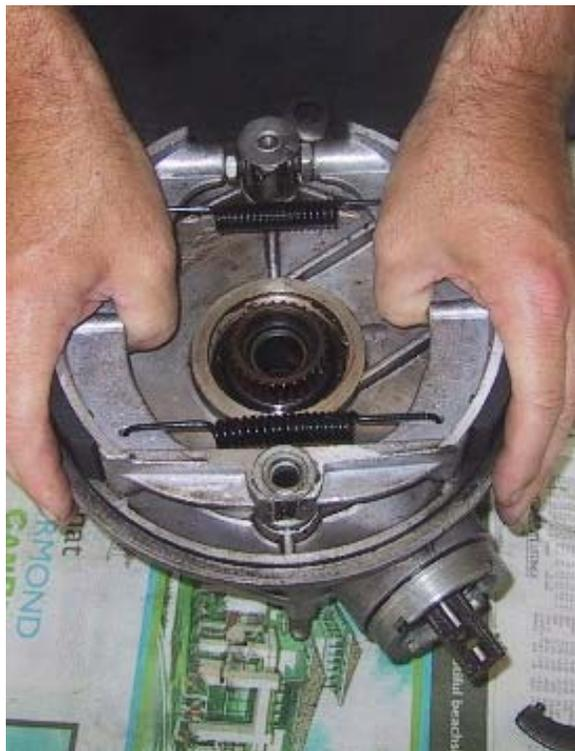
To remove the brake shoes from any drum, grasp the middle of the shoe with your thumbs...
