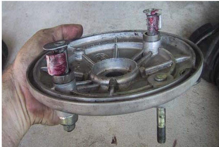
**After cleaning the brake parts, grease the two brake cams and contact surfaces of the brake shoes.**
