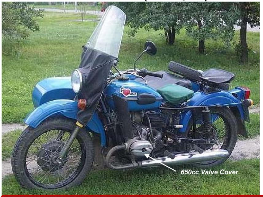
Notice the single bracket on the front fender and the bottle-cap wheel hubs
