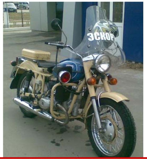
Irbitsky plant produced special "Ural" - Patrol IMZ-8.923's for the GAI, with a set of flashing lights, mechanical siren and other special devices.
