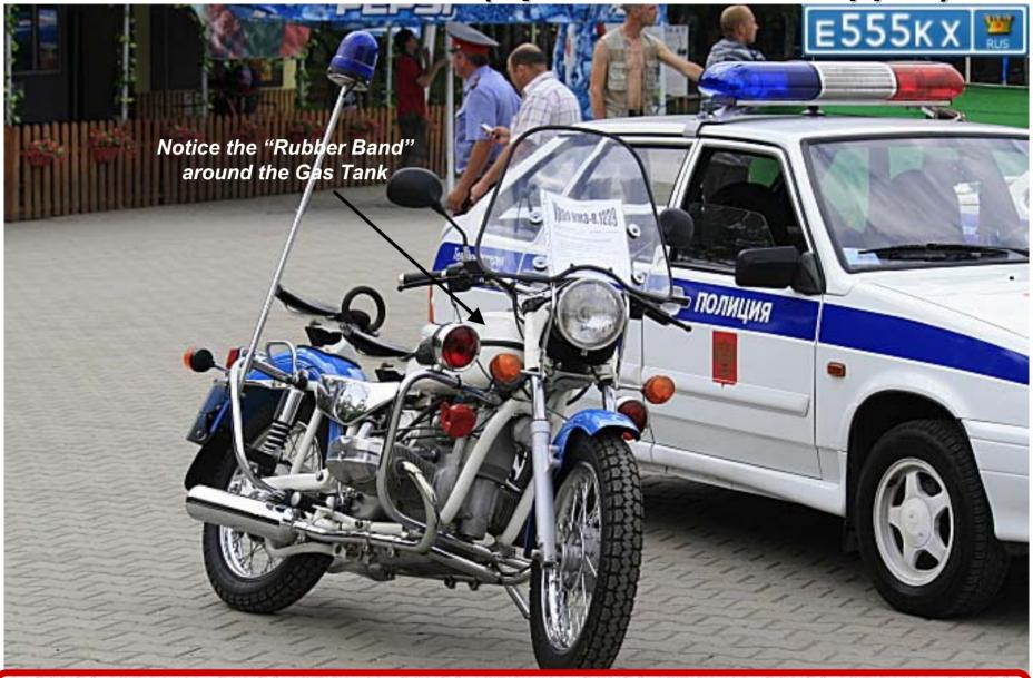
The police (DPS) version of the solo motorcycle was based on the commercial version, with the addition of a special wind shield, signal lights and siren. 8
