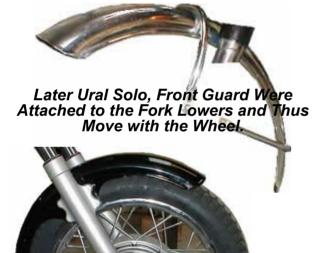
The latest 750cc solo bikes have changed to Paioli forks, with new fork mounted mudguard. The brake and wheel are the same but the spindle is very different.
