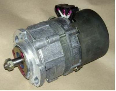
The *C-424* alternator surfaced in 1974 on Ural's M-67 and Dnepr's MT-10, as Russian motorcycles migrated to 12-Volts.
