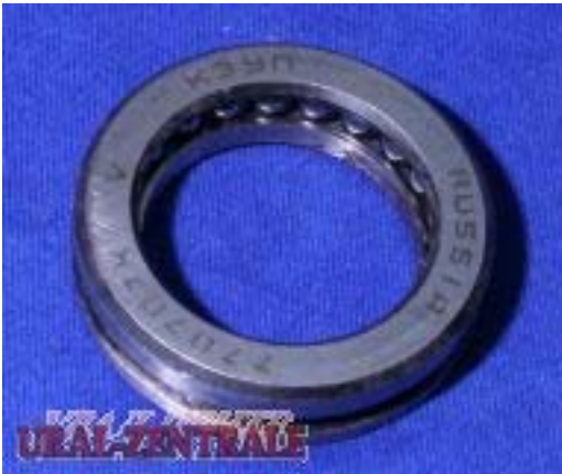
Steering Head Bearing for Dnepr /Ural / K-750 / M-72, etc. original design, 1 bearing complete with lower and upper shell and balls Product ID: S878 List Price: €8.49
