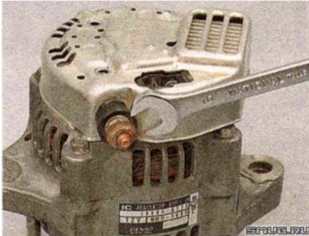
15. Using a 10 mm Open-End Wrench, Loosen Two Nuts on the Positive Terminal of the Alternator.
