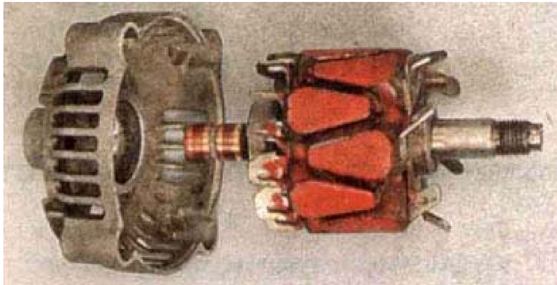
34. Check the Condition of the Rear Bearing, Its Rotation Should Be Smooth, Without Play, with Negligible High-Speed Rotational Noise. If Needed, Use a Standard Pulley-Puller to Remove the Defective Bearing from the Shaft and Replace It.
