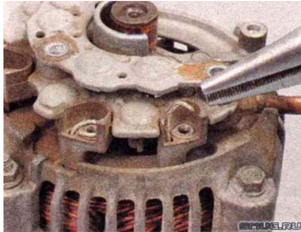
24. Access to the Ends of the Alternator Windings Under the Screw Heads Is Accomplished by Removing the Screws. Use Pliers to Straighten Them. This Must Be Done Very Carefully, So As Not to Damage the Ends.
