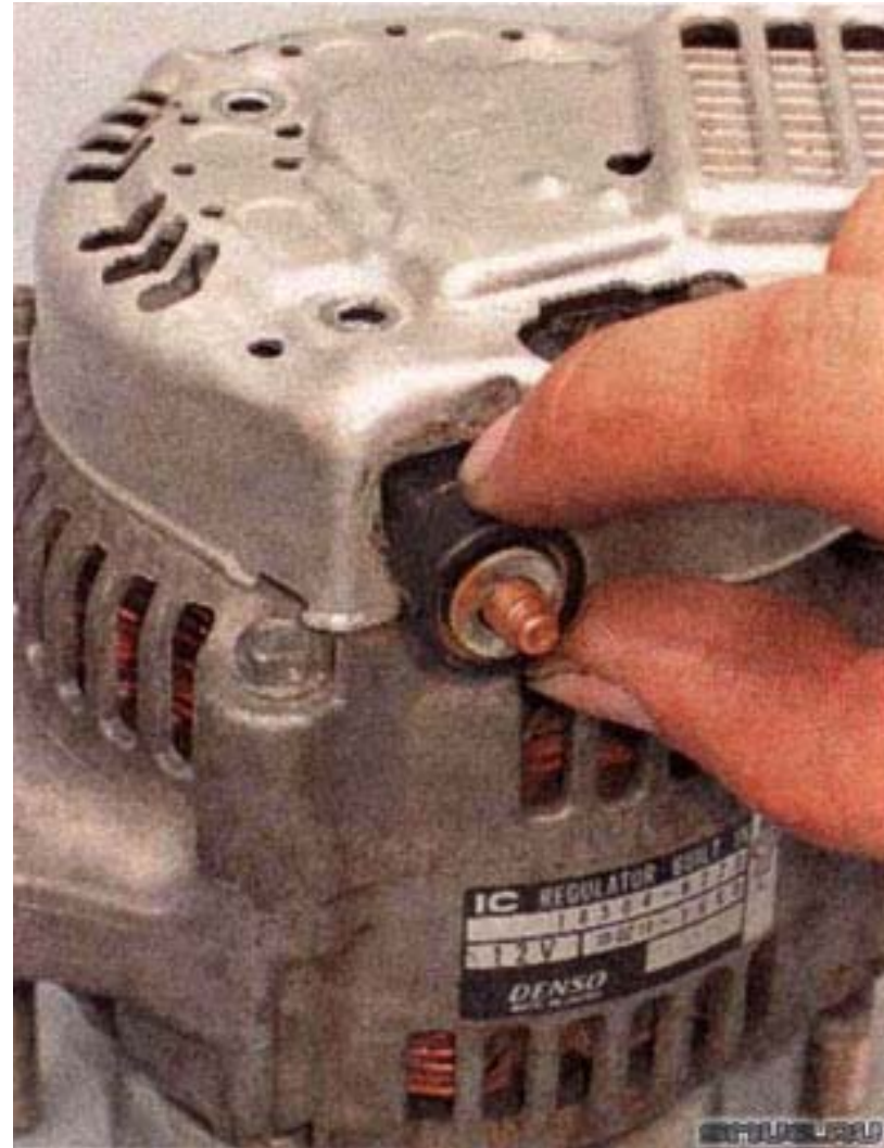
16. Remove the Plastic Grommet from the Body.
