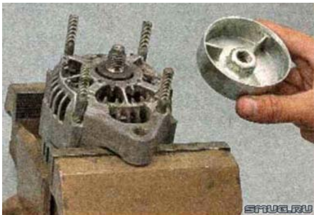
28. Remove the Clip Damper, Underneath Which Is a Remote Bushing.
