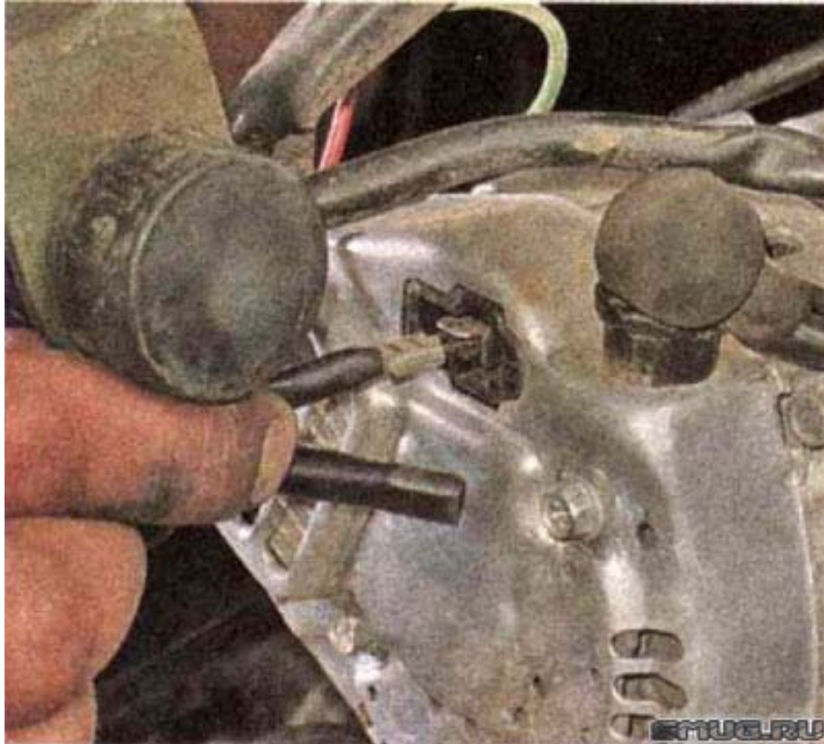
1. Disconnect Two Wires from Terminals on Back Cover of the Alternator.
