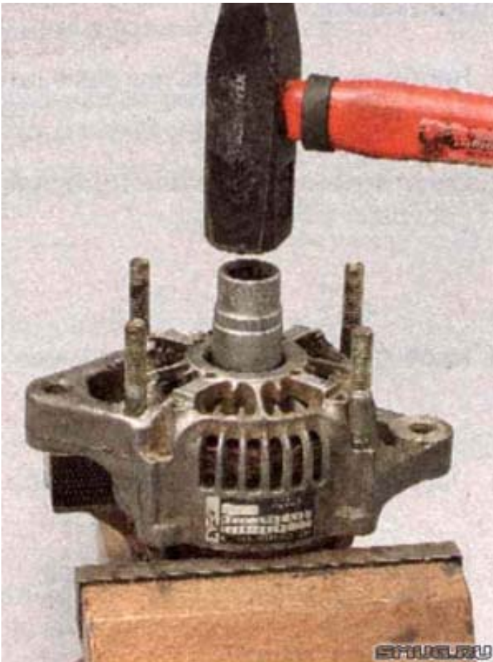
33. A 19 mm Ratchet Socket or Mandrel Is Used to Extract the Front Bearing.
