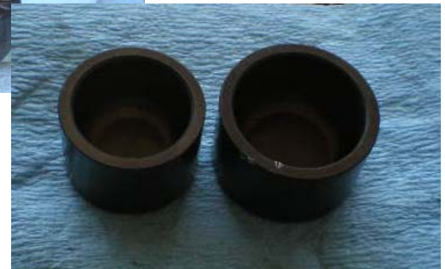
Two of the pistons...there are four (2) 30mm & (2) 34mm pistons
