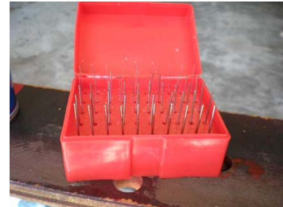
Pin set used to clean the small openings in the carb too.
