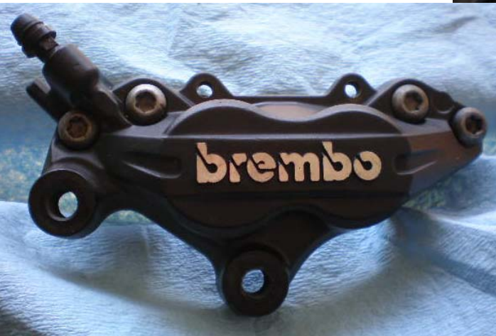
Note the 4 bolts securing the Brembo caliper halves
