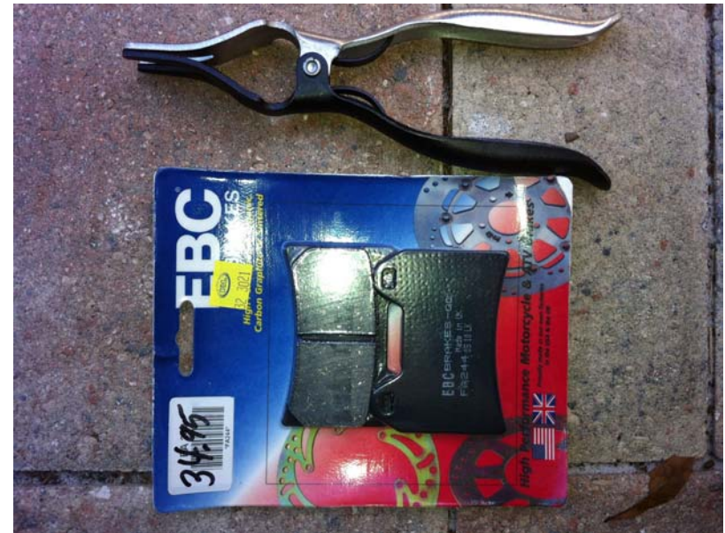
The tool is for rubber hose removal but works great for spreading brake pucks.
