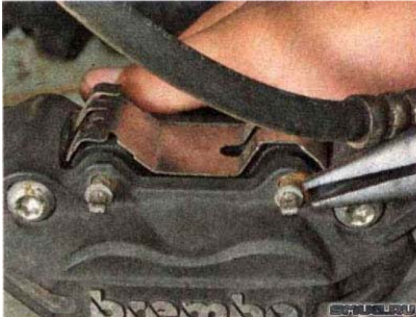
4. Pliers pull out the two guides, brake pad out of the caliper.
