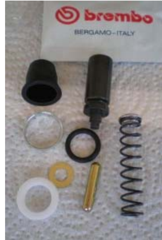
All the component needed plus the lubricant that came with the kit. Note the O-ring, seal (white), & seal retaining ring (silver)...these go into the BMC bore.
