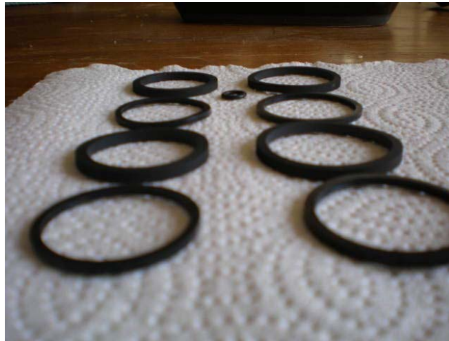
Note that the bottom seal is thicker than the top (wiper) seal.
