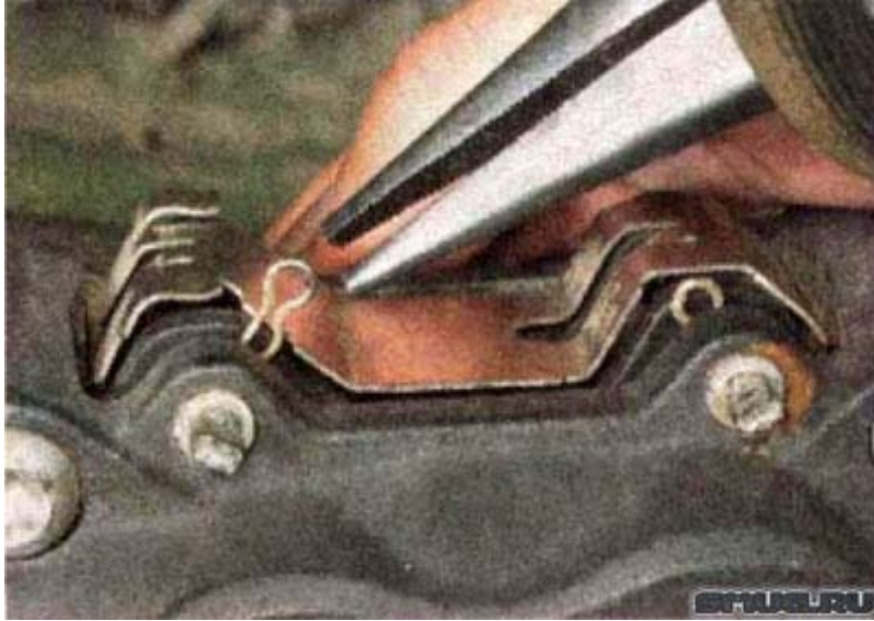
3. Tweezers pliers and pull out two cotter pin securing the caliper.
