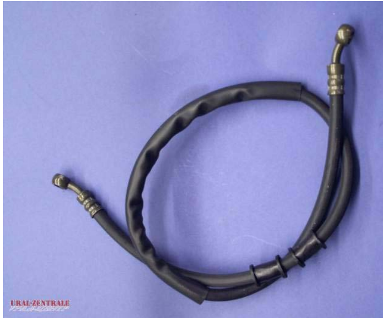
Early Rubber Brake Hose for Disc Brake Product No.: S2073-S Manufacturer: SASIC FRANCE Length: 96 cm Pressed-on 10 mm Banjo Fittings with Protecting Tube List Price: 11.89 EUR ( www.ural-zentrale.de )
