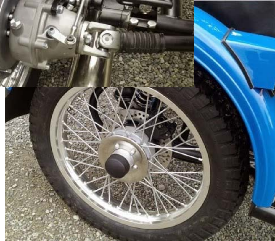
Brembo Disc Brake with 2-Piston Caliper and NG Floating Disc
