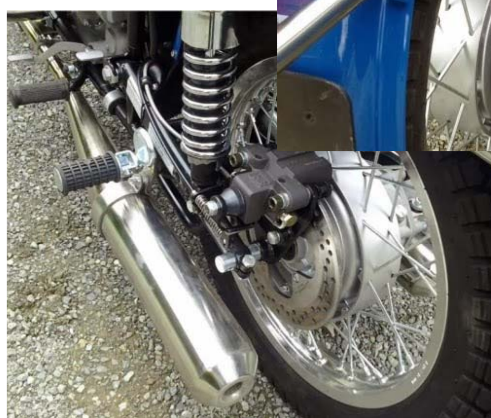
Rear Disc (hydraulic + mechanical) Hayes Brakes with Single-Piston Floating Caliper and Integrated Parking Brake
